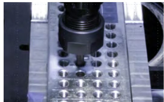
Tapping Torque Test Setup
