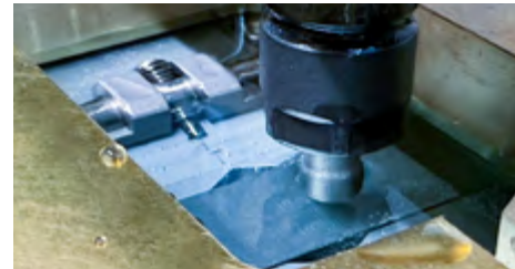
Pin-on-Plate with lubricant
